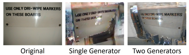
Figure 2. Using a single generator to achieve completion and appearance adaptation will introduce blur as shown in ‘Single Generator’. The use of two sub-generators improves the quality of the adapted image significantly as shown in ‘Two Generators’.
