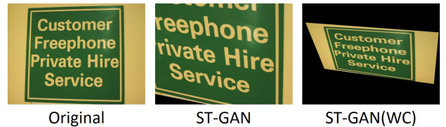
Figure 3. The ST-GAN will lose the border region. So we constraint the range of the transformation parameters as predicted by the ST-GAN in the test phase, so that the transformed image can preserve all the information of original image as shown in ST-GAN(WC).
