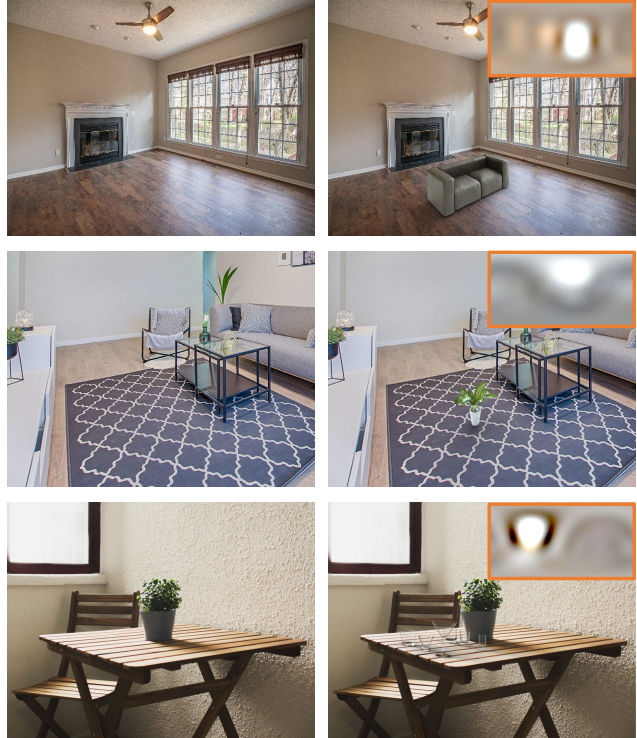
Figure 7. Object relighting on a variety of photos from the Internet. In all cases, light estimation is performed completely automatically by our model. The predicted illumination maps are utilized to relight the virtual objects with Blender [9]. More rendering samples and the analysis of spatially-varying rendering are available in supplementary file.
